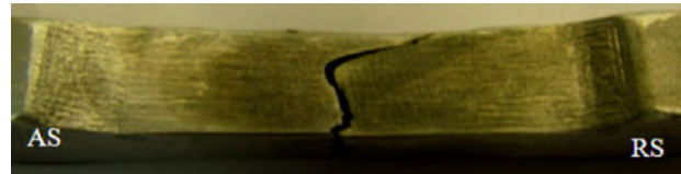
Fig. 13 Location of fracture (from boundary of SZ and TMAZ) after tensile testing
