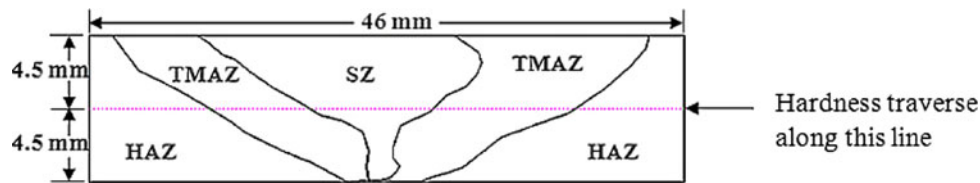
Fig. 11 Schematic diagram for microhardness traverse position
